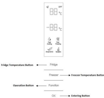
**TEMPERATURE SETTING:** Click the "Fridge" or "Freezer" button and when it flickers in the symbol, temperatures can be set. Each time when the button is clicked, the temperature changes accordingly. Temperatures cannot be set under functions of fast cooling, fast freezing, Smart ECO and vacation. Under temperature setting, if there is no button operation in 5 seconds, the button stops flickering and the set temperature comes into effect.
