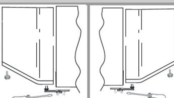
Remove the middle screw and remove the top door
