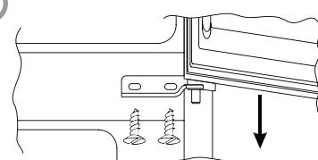
Remove the caps (A) and (B), loosen the screws and partially remove the panel.
