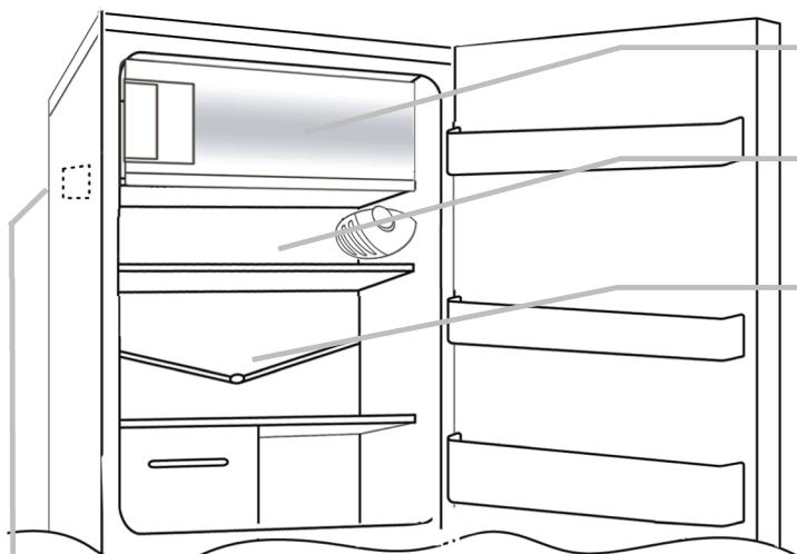
We recommend you defrost the freezer area when the layer of frost is more than 3 mm thick.
