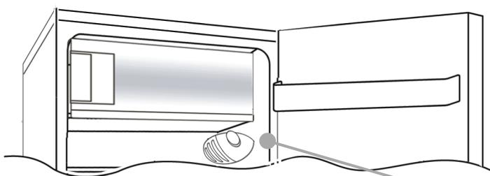
The thermostat box to control the appliance is located inside the fridge compartment on the top right. To check whether the appliance is functioning, make sure that the thermostat knob is not set on **0°**.
