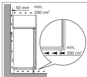
Level the appliance using the adjustable feet, ensure there is a gap between the bottom edge of the appliance and the ground, so that there is sufficient circulation of the cooling air, by which you will ensure the optimal performance of the cooling circuit.
