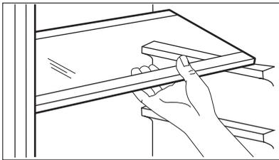
The walls of the refrigerator are equipped with a series of runners so that the shelves can be positioned as desired. For better use of space, the front half-shelves can lie over the rear ones.
