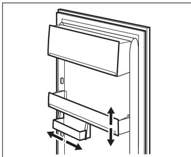
To permit storage of food packages of various sizes, the door shelves can be placed at different heights. To make these adjustments proceed as follow: gradually pull the shelf in the direction of the arrows until it comes free, then reposition as required.
